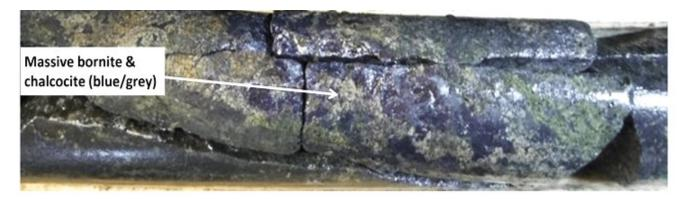
Now hold on to your hat. I want to show you what is important about all this black you see in Zonte's drill core. It is Chalcocite, a secondary copper mineral that forms from the <u>weathering</u> of primary sulfide minerals, such as chalcopyrite. **It contains up to 80% copper by weight** and is an important source of copper in some deposits.
