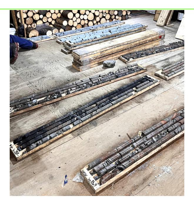
Chalcocite is the highest grade copper mineral and that is what you see in this drill core. That said, we don't know if there is enough chalcocite distributed throughout the core for high grade assay results. There is no telling for sure if we see 0.2% copper over many meters or 15% copper. We have to wait for assays.
